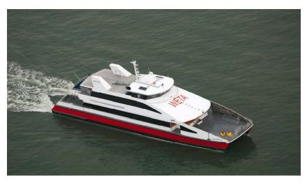
**∢WETA's** Gemini and Pisces ferries are among the nation's most environmentally responsible passenger vessels. The engines surpass Tier II emission mandates, is has solar panels, operates on a blend of biodiesel and ULSD fuel, and its hull is designed to
