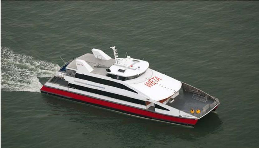
◀WETA's Gemini and Pisces ferries are among the nation's most environmentally responsible passenger vessels. The engines surpass Tier II emission mandates, is has solar panels, operates on a blend of biodiesel and ULSD fuel, and its hull is designed to
